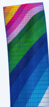
Fig-2: Finite element showing regular cylindrical implant with maximum displacement of 8.5 Micron.
